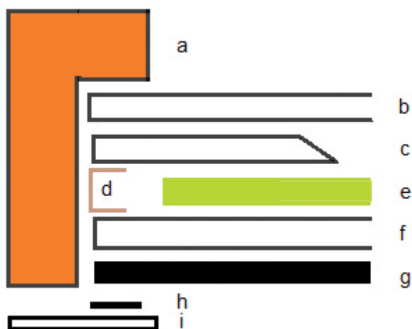
Diagram 1: Cross section of a framed work on paper showing the relationship of the components inside the frame
